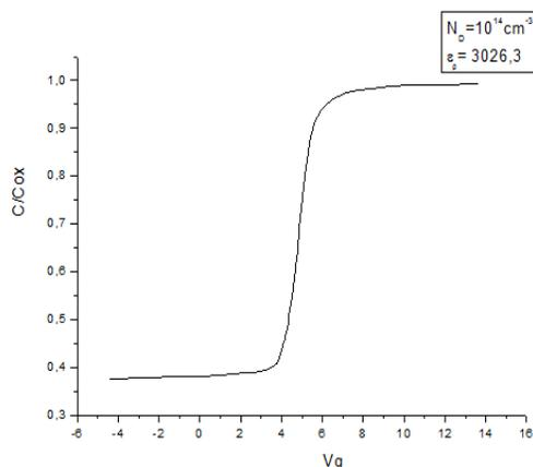
**Figure No. 3: Total Capacitance of the Structure with Blood in Place of Airgap.**
