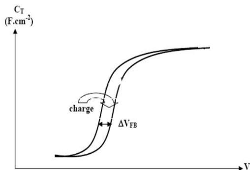
**Figure No. 4: Effect of the Absorption of Charges on the Interface [7].**
